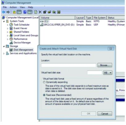
DiskManagement Tool: With the ability to create and attach virtual hard drives from the GUI
